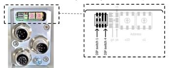
The device controls and status elements are located under the sealing plug. You will need a nonconducting pointed object to adjust the switches.
