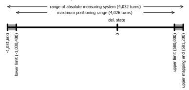
Here, the upper mapping end was decreased from the value 806,400 to 581,200. Consequently, a higher proportion of the possible positioning range is in the negative range and a smaller proportion in the positive range.
