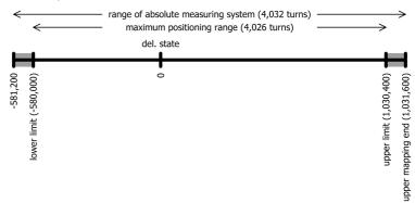
Here, the upper mapping end was increased from the value 806,400 to 1,031,600. Consequently, a higher proportion of the possible positioning range is in the positive range and a smaller proportion in the negative range.
