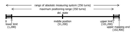
In the delivery state, the values from the following table result for the upper mapping end and the lower and upper limits:
