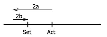
3. New setpoint position is only slightly larger than the current actual position and previously there was no positioning movement with loop (e.g. a manual movement):
