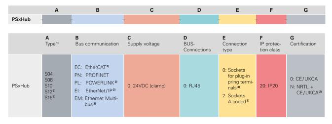
$<sup>^{11}\,\</sup>mathrm{S}$  stands for the control cabinet variant, the numerical value for the number of ports
