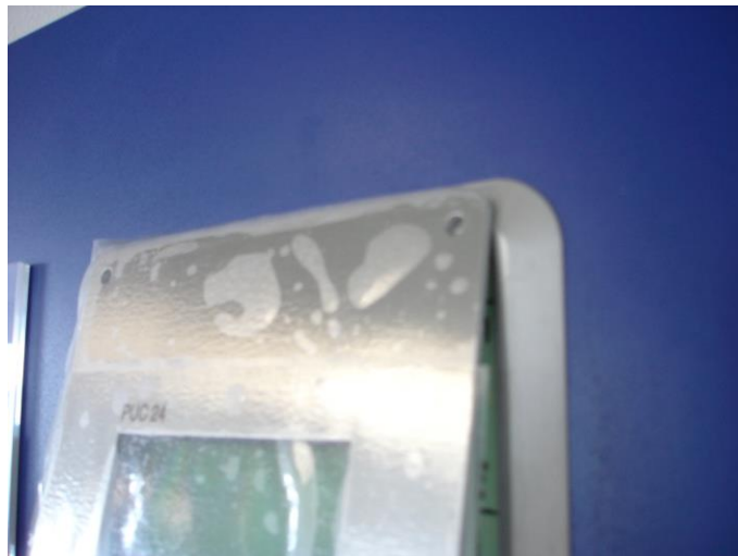
Fig. 10: Slide the PUC 24 upwards into the mounting frame and pivot into place
